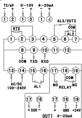
when AI708-4 input 4~20mA, should change signal manually
