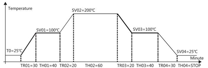
Note: cooling rate of the curve can't be faster than the natural cooling rate of the controlled object.
