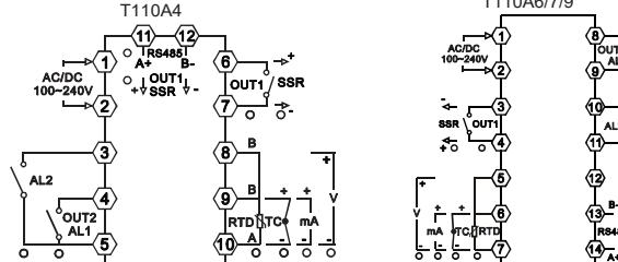
Note: In actual wiring diagram, solid circles indicate have the function, while hollow circles means no this function. Solid or hollow dots will be marked according to the actual function.
