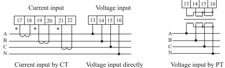
Mode 2(2pcs CT): 3phase 3wire connection(For Kwh)
