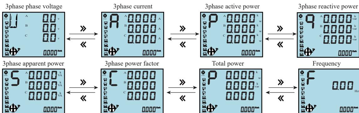
Illustration for measure interface switch procedure:
