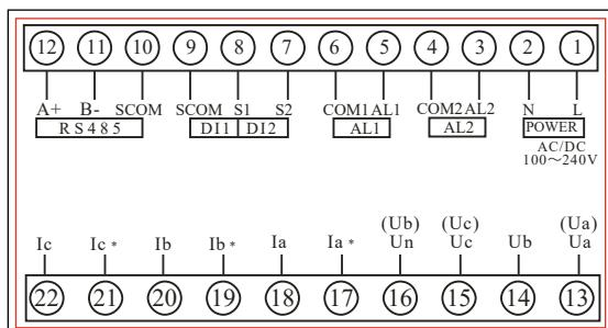
Note: Voltage input connection terminal, labels in bracket show 3 phase 3 wire connection method;
